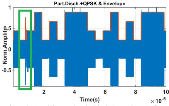
Figure 2. PD+COMM signals (blue) & envelope (red).
