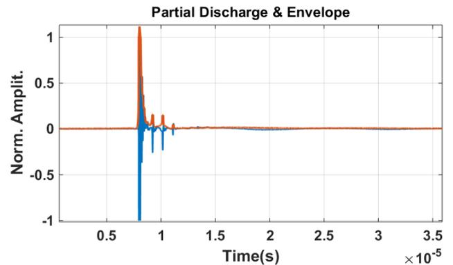
Figure 1. Partial discharge (blue) & envelope (red).
