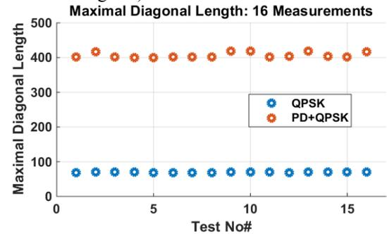
Figure 12. Results for 16 PD/PD+COMM pairs of signals: maximal diagonal length.
