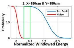
Fig. 10. Survivor function for the  $2^{nd}$  configuration: Probability of detection (Arc Fault – Blue) & Probability of false alarm (Noise – Red) vs. Normalized Threshold, Range of Thresholds with 0% false alarms & 100% detection – Green rectangle.
