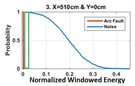
Fig. 11. Survivor function for the 3<sup>rd</sup> configuration: Probability of detection (Arc Fault – Blue) & Probability of false alarm (Noise – Red) vs. Normalized Threshold, Range of Thresholds with 0% false alarms & 100% detection – Green rectangle.
