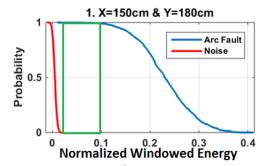
Fig. 9. Survivor function for the 1<sup>st</sup> configuration: Probability of detection (Arc Fault – Blue) & Probability of false alarm (Noise – Red) vs. Normalized Threshold, Range of Thresholds with 0% false alarms & 100% detection – Green rectangle.
