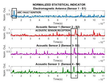
Fig. 7. Aggregate statistical indicator (normalized) example for a set of signals (one measurement).
