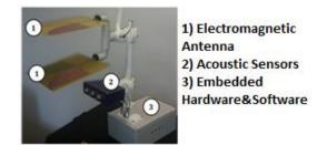
Fig. 2 Description of the detection and localization system.
