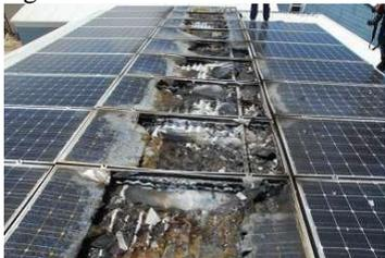
Fig. 1 DC arc fault in a photovoltaic system [4].
