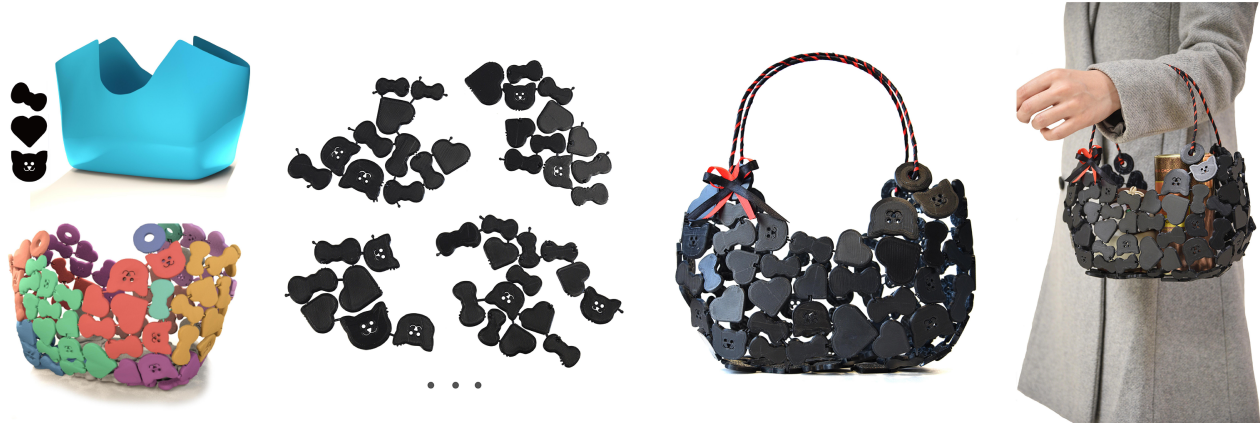
Fig. 1. Given a target surface and a set of user-specified tiles (top left), our method produces a dedicated packing of tiles that is optimized for fabrication (bottom left). The results are printed as independent flat patches (second column) with integrated hinges and snap-fit joints. The patches are folded and assembled into the final object (third column); in this case a functional handbag that can carry light objects.
