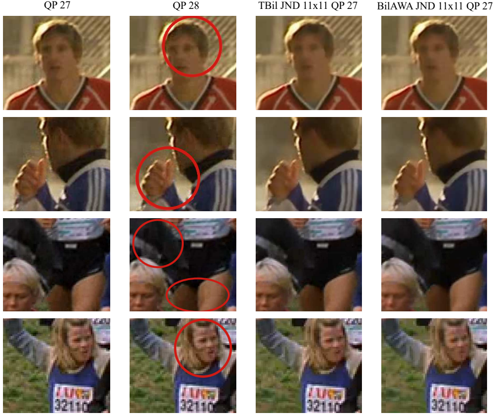
Figure 1. Comparison between coarser quantization and pre-filtering: the first and second lines show zoomed areas from the Soccer sequence, the third and fourth lines from the CrowdRun sequence. In the first column, the content has been encoded with H.264/AVC (QP=27, IBBP12). Encoding with coarser quantization QP=28 leads to a bitrate reduction of 13.5% for the Soccer sequence and of 12.9% for the CrowdRun sequence, but at the expense of visible blocking effect in the reconstructed image (second column, see areas circled in red). In comparison, our perceptual pre-filtering introduces a slight blur which is much less annoying than blockiness for the end user, for a similar bitrate reduction: \Delta\text{Bitrate} = -9.2\% for the Soccer sequence and \Delta\text{Bitrate} = -7.4\% for the CrowdRun sequence (third column). \Delta\text{Bitrate} = -16.0\% for the Soccer sequence and \Delta\text{Bitrate} = -14.2\% for the CrowdRun sequence (fourth column).
