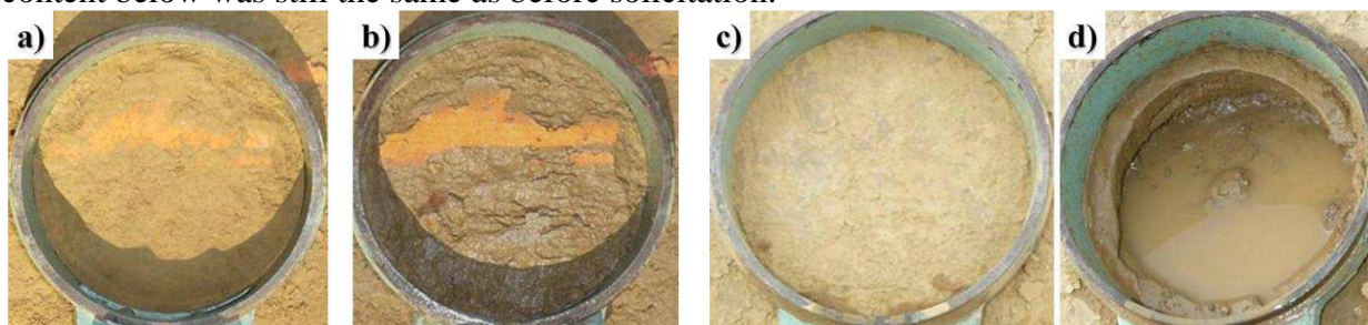
Figure 9. Soil surfaces before and after normal protocol MoJET tests, 28 days after the construction. Soil treated before test (a) and after test (b); untreated soil before test (c) and after test (d).
