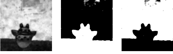
Fig. 3. Separation on two depth planes: depth map (the left column) and the weights w^1 and w^2 associated to each depth plane (the middle and the right columns).
