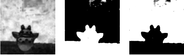
Fig. 3. Separation on two depth planes: depth map (the left column) and the weights w^1 and w^2 associated to each depth plane (the middle and the right columns).
