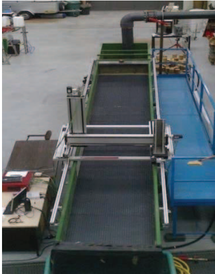
Fig. 1. Open channel flume used in experiments (IMFT, 2015).
