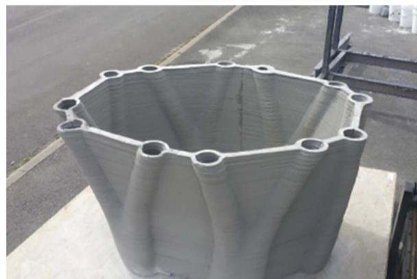
Fig. 3. Mould for a space truss (XtreeE, 2016).
