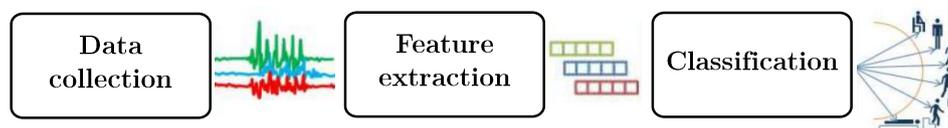
Figure 1: General structure of a HAR process
