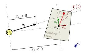
Fig. 1. **Definition of the inertial frame**  $(e_x, e_y, e_z)$ . The frame is rooted at the stationary CoP location  $r_f$ . The instantaneous CoM location is denoted by  $c_i$ . Both vectors  $e_x$  and  $e_y$  lie in the horizontal plane, and  $e_x$  is aligned with the (horizontal projection of the) desired direction of motion  $r_f - c_i$ .
