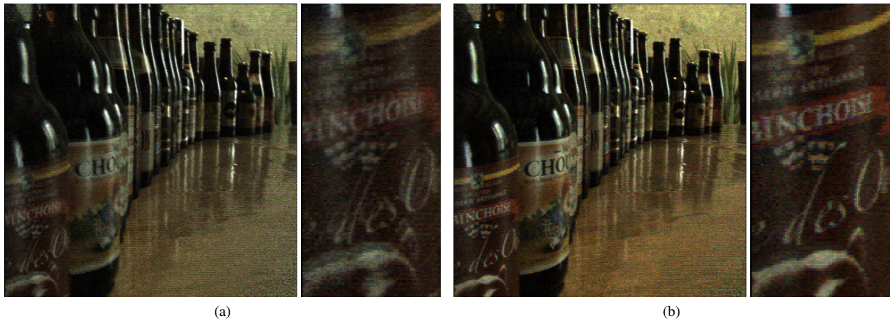
Fig. 11. Extracted peripheral view from a real lenslet image taken with a Lytro 1: (a) is decoded as described in [11], (b) is decoded with our proposed demosaicing and alignment methods.
