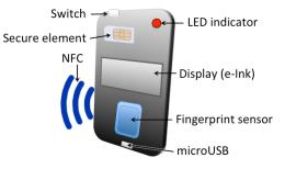
Figure 1: OffPAD v.1 design elements
