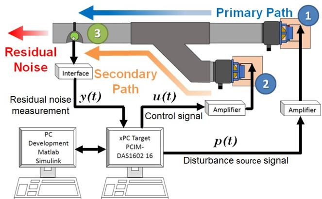
Fig. 2. Duct active noise control test bench diagram.
