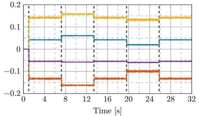
Fig. 16. Evolution of the parameters of the adaptive controller in the presence of step changes in disturbances frequencies.
