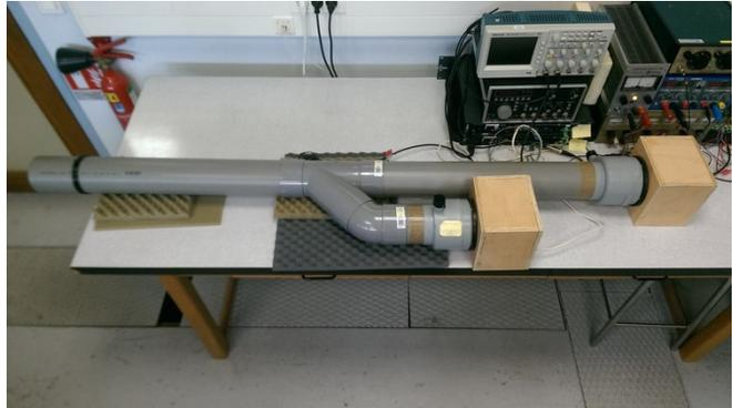
Fig. 1. Duct active noise control test bench (Photo).
