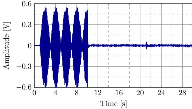
Fig. 9. Acoustic interference attenuation using an adaptive controller. Noise frequencies: 170+170.5 Hz, 285+285.5 Hz then 180+180.5 Hz, 295+295.5 Hz. Loop closed at 10s.
