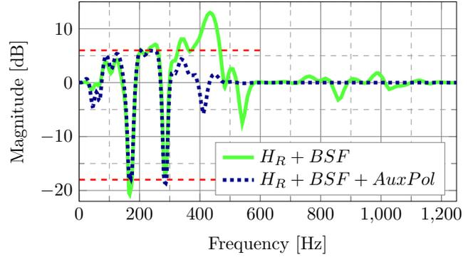
Fig. 5. Robust controller design, Output sensitivity function evolution.
