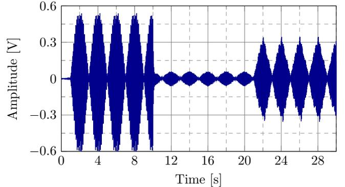
Fig. 8. Acoustic interference attenuation using a robust controller. Noise frequencies: 170+170.5 Hz, 285+285.5 Hz then 180+180.5 Hz, 295+295.5 Hz. Loop closed at 10 s.
