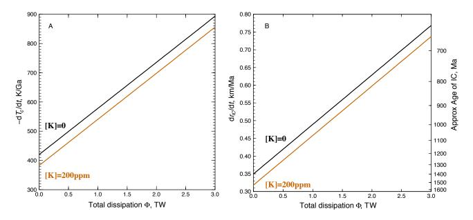
Figure 3: Core cooling rate just before the onset of inner core crystallization (A) and present inner core growth rate (B) as function of total dissipation. Also given on the right axis of B is the approximate age of the inner core, in Myr. See § 3.4 for details of this calculation.
