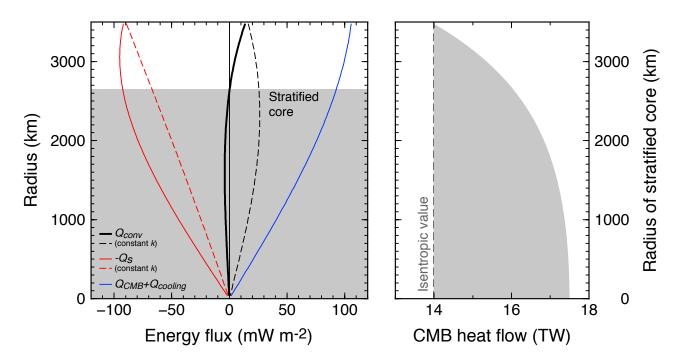
Figure 10: Radial profiles of contributions to the convective heat flux density (A) and limit to the region with negative convective heat flow as function of the CMB value (B) for the period just preceding the onset of inner core crystallization. The profiles are computed for  $Q_{CMB} = 16.1$ TW for an isentropic value  $Q_S = 14TW$ . The dashed lines are obtained for constant value of the thermal conductivity, equal to the CMB value, and show no stratification.
