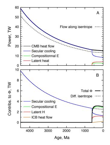
Figure 11: Evolution of the contributions to the the CMB heat flow (A) and total dissipation (B) as function of time for a CMB heat flow that is always 1.15 times the isentropic value.
