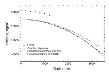
Figure 1: Density as function of radius in the core. Circles are the PREM values, the solid line is the 4<sup>th</sup> order fit according to equation (5) with parameters given in table 2. The dashed line and dash-dotted line are exponential forms  $\rho = \rho_0 \exp(-r^2/L^2)$  using L = 7765km and L = 7400km, respectively.
