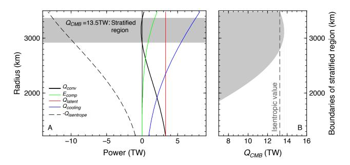
Figure 8: Radial profiles of contributions to the convective heat flow (A) and limits to the region with negative convective heat flow as function of the present time CMB heat flow value (B). The profiles are computed for  $Q_{CMB} = 13.5$ TW, that is slightly larger than the isentropic value ( $Q_S = 13.25$ TW).
