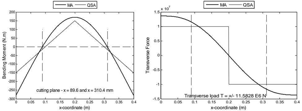
Fig. B.1. Bending moment (left) and transverse force (right) belonging to the cross sections of the beam studied. The dashed lines indicate the cutting planes located at  $x = 100$  and  $300$  mm under the quasi static assumption and at  $x = 89.6$  mm and  $310.4$  mm under the modal assumption. These results were obtained considering a analytical beam model under a Timoshenko assumption.
