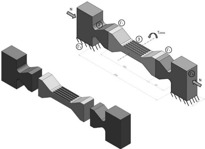
Fig. 1. View of the specimen. On the left: the three parts of the beam. On the right: the testing device assembled. Faces  $\Gamma_U$  are screwed on an anti-vibration marble. Strain gauges are glued on both sides (2) of the beam to measure the normal load. Piezoelectric patches (3) are glued on both sides of the beam to apply a torque  $T_{piezo}$  to excite the first vibration mode. A quick clamp is used to apply the normal load before the tests on faces  $\Gamma_N$ .
