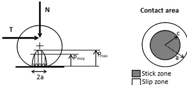
Fig. 4. Schematic elastic spheres pressed by a constant normal force  $N$  and subjected to an oscillating tangential force  $T$ .
