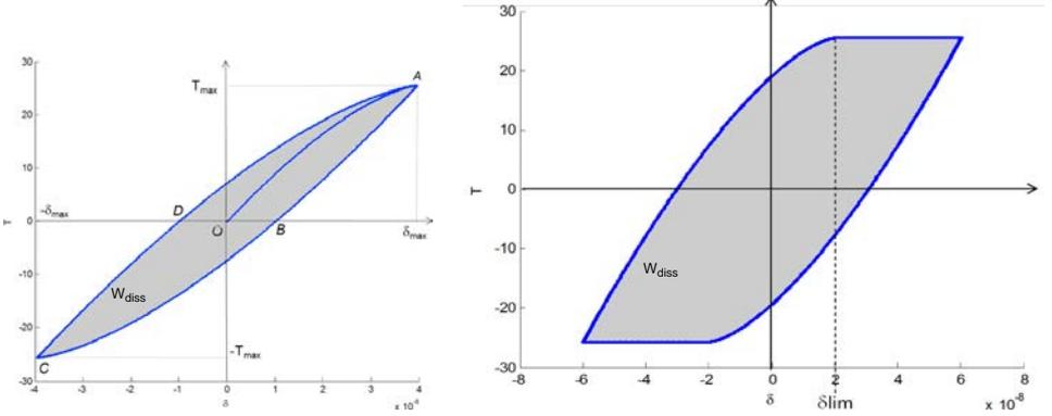
Fig. 5. Left: Loading cycle with partial slip for one spherical contact. Tangential load  $T(N)$  versus  $\delta$  displacement in the contact (m). Right: Loading cycle with macro-slip for one spherical contact. Tangential load  $T(N)$  versus  $\delta$  (m) displacement in the contact.
