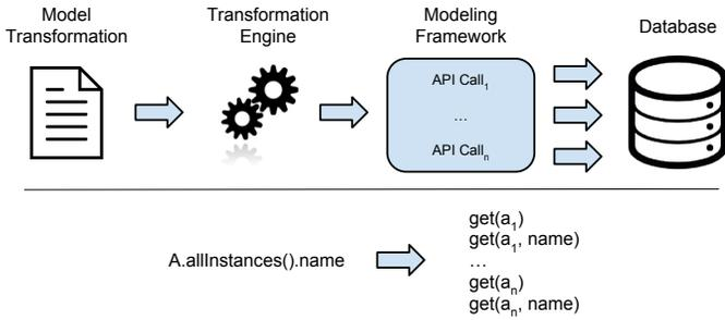
Fig. 1. Model Transformation Engine and Modeling Framework Integration
