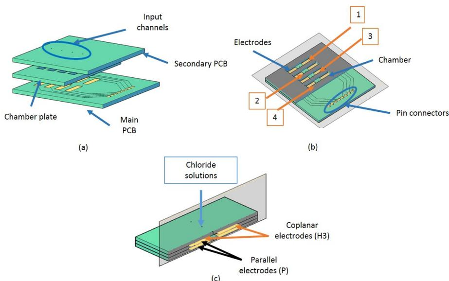
**Figure 9.** (a) sensor design; (b) longitudinal section of the device showing the label for each chamber; and (c) cross section of the third chamber showing the label of each capacitor according to the chamber.
