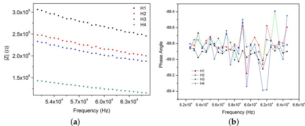
**Figure 10.** Bode diagrams of coplanar plates capacitors of empty device (NCA) (a) Impedance and (b) Phase angle.
