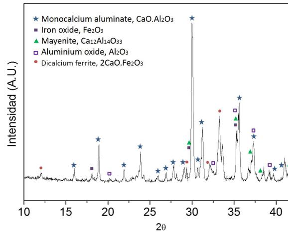
**Figure 4.** XRD Spectrum of Aluminate Ternal RG.
