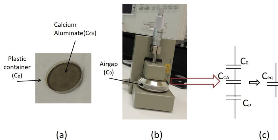
**Figure 3.** (a) CA sample in the container; (b) Sample located in the Dielectric test fixture 16451B; (c) Equivalent circuit ( $C_e$ ).
