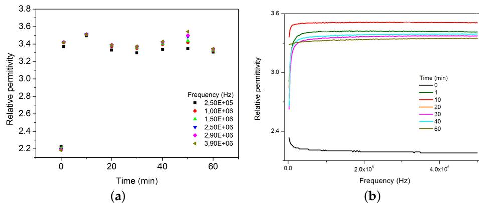
**Figure 5.** Time effect on CA's behavior when 0.7 M NaCl solutions are added at specific frequencies. (a) Relative permittivity vs Time, regarding specific frequencies and (b) Relative permittivity vs. Frequency, regarding time. At 0 min the CA was dried.
