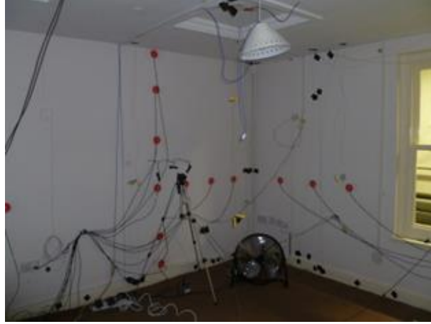
Figure 1 - Photograph of bedroom 1 in the test house showing HFPs (red discs) on the thermal elements
