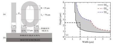
Figure 1: Schema of a top view (a) and a cross section (b) of the porous silica racetrack MR. (c) Solutions of the Maxwell equations for the  $TE_{00}$ ,  $TE_{01}$  and  $TE_{10}$  modes as a function of the porous silica ridge waveguide dimensions.
