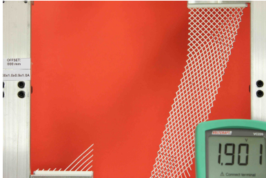
(C) . Sample A after complete failure.
