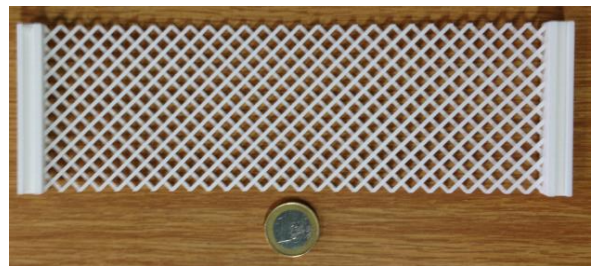
FIGURE 1. Example of a pantographic structure developed by [2].
