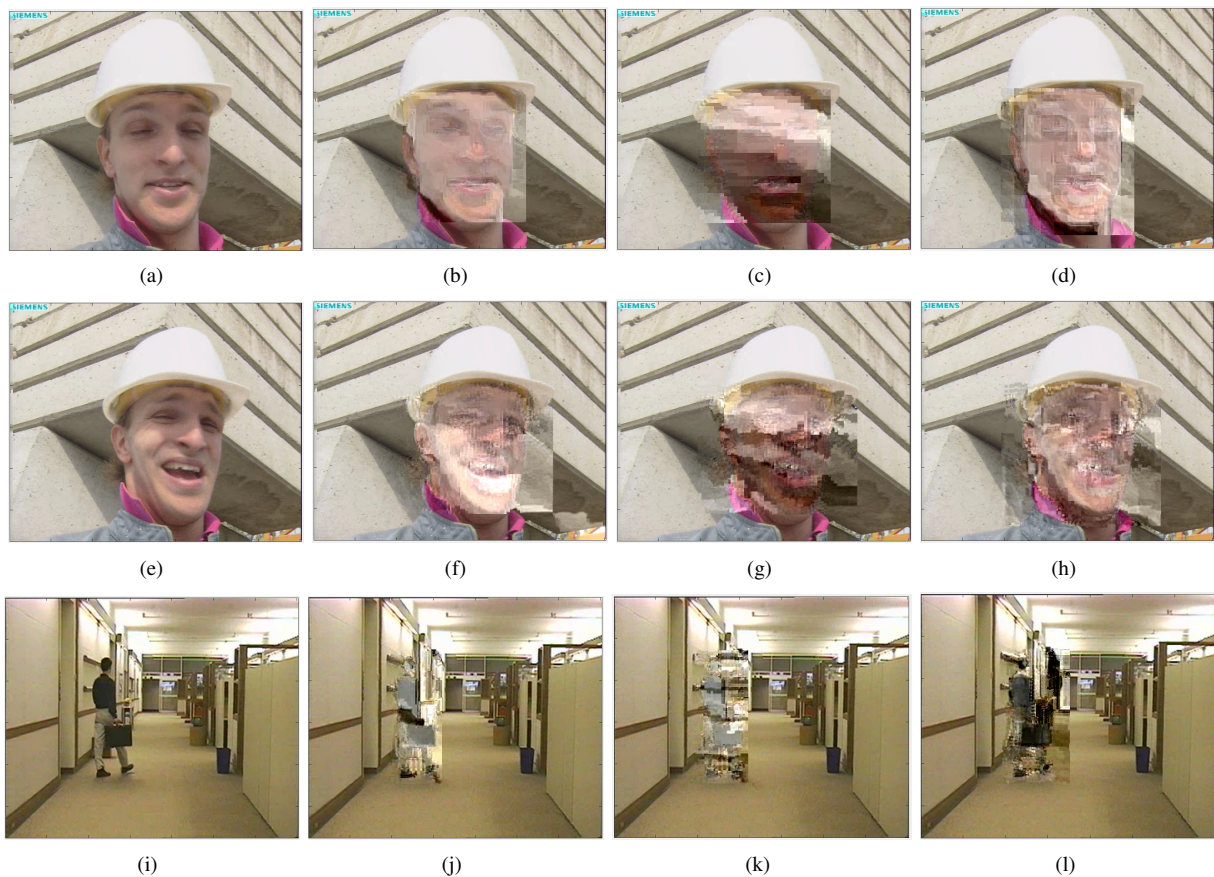
Fig. 2: With CIF size, QP=24 and IP=5 : (a) The 1st frame of original 'foreman' (I frame), (b) encrypted by SNC, (c) encrypted by SNC+IPM, (d) encrypted by our process. (e) The 15th frame of original 'foreman' (P frame), (f) encrypted by SNC, (g) encrypted by SNC+IPM, (h) encrypted by our process. (i) The 40th frame of original 'hall' (P frame), (j) encrypted by SNC, (k) encrypted by SNC+IPM, (l) encrypted by our process.
