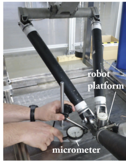
(a) Micrometer for measuring the repeatability
