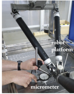
(a) Micrometer for measuring the repeatability
