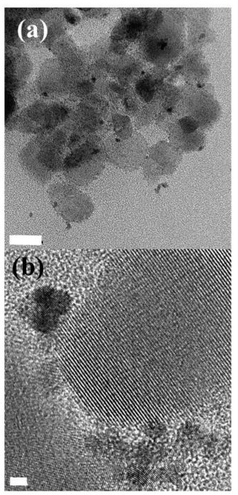
**Figure 8.** (a) TEM image of platinum nanoclusters generated in a selective way on nano- $TiO_2$  by exposure for 90s simultaneously to 50% UV light intensity and an electric field of 3kV/m. (b) HRTEM image for a typical deposit obtained under these conditions, zooming on the junction between the metal nanocluster and a nano- $TiO_2$  particle (scale bars are 20 and 2 nm respectively).
