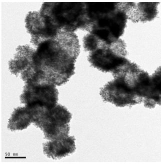
**Figure 7.** TEM image of nano-TiO<sub>2</sub> particles covered with platinum nanoclusters generated in an unspecific way by exposure for 90s to 50% UV light intensity.
