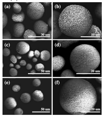
**Figure 4.** Asymmetric gold deposited on micro-TiO<sub>2</sub> obtained for simultaneous exposure for 30s to 20% UV light intensity and an electric field of (a-b) 33kV/m (c-d) 17kV/m and (e-f) 3kV/m.
