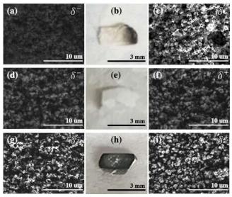
**Figure 3.** Deposition of platinum on macro-TiO<sub>2</sub> particles. (a-c) For simultaneous application of an electric field (E) and UV light, SEM images show no platinum on the  $\delta^-$  side and platinum particles (white spots) on the  $\delta^+$  side; (d-f) No metal deposition is observed when only an electric field is applied; (g-i) Non-specific metal deposition is obtained when only UV light is used but no electric field.
