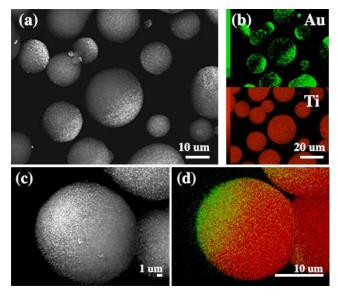
**Figure 5.** (a) and (c) SEM images of gold deposited on micro-TiO<sub>2</sub> by a simultaneous exposure for 30s to 20% UV light intensity and an electric field of 3kV/m. (b) and (d) EDX analysis of (a) and (c) respectively, red colour for Ti and green for Au.
