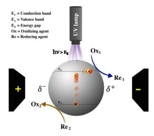
Figure 1. Schematic mechanism of metal deposition on TiO<sub>2</sub> particles.
