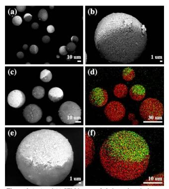
**Figure 6.** (a-c) and (e) SEM images of platinum deposited asymmetrically on micro-TiO<sub>2</sub> by a simultaneous exposure for 90s to 50% UV light intensity and an electric field of 3kV/m in a solution containing 5 mM H<sub>2</sub>PtCl<sub>6</sub>.xH<sub>2</sub>O; (d) and (f) EDX analysis of (c) and (e) respectively, red colour for Ti and green for Pt.
