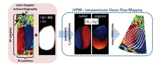
**Figure 2.** The *i*VFM algorithm is based on an automatic  $\ell_2$ -norm minimization. It works in a polar coordinate system, before scan conversion.  $\Omega$  represents the domain of interest and  $\partial\Omega$  is its boundary.
