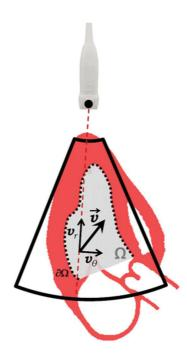
**Figure 1.** The *i*VFM algorithm was implemented in the polar coordinate system associated with the Doppler sector. *i*VFM allows one to recover the 2D velocity field  $\vec{v}(r,\theta)$  from the Doppler components by minimizing the cost function described by equation (2).  $\Omega$  represents the domain of interest and  $\partial\Omega$  its boundary.
