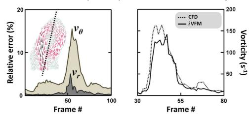
**Figure 6.** Analysis in the patient-specific CFD heart model. Left panel: comparison between the iVFM-based and CFD velocity vectors. The radial and angular components were compared on the apex-mitral axis (dotted line of the inset). Right panel: comparison of the peak vorticities.
