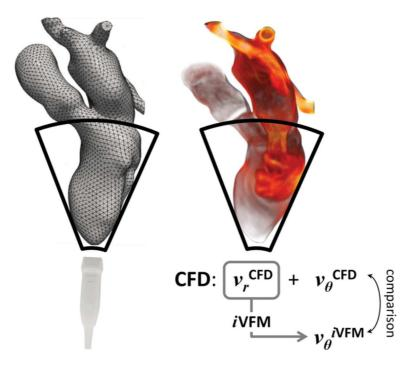
**Figure 3.** The *i*VFM algorithm was tested in a dynamic patient-specific heart flow model (Chnafa *et al* 2014). Doppler velocity images were simulated from the radial velocity components. The vector fields recovered by *i*VFM were compared with the ground-truth CFD fields.
