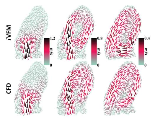
**Figure 5.** Analysis in the patient-specific CFD heart model: comparison of the intraventricular velocity vector fields (*i*VFM-based vectors versus original CFD vectors). These snapshots correspond to frame numbers 50, 60, and 70 (see figure 6).
