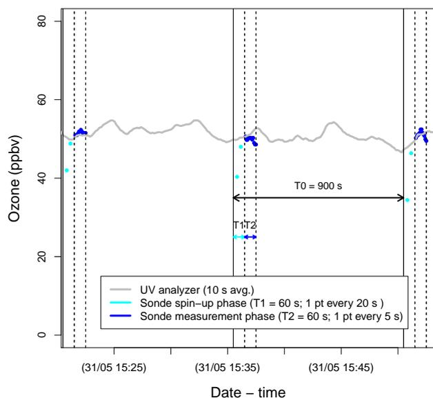
**Figure 3.** Example (taken from the laboratory test detailed in Sect. 3.2) showing three measurement cycles of the BLPB ozonesonde. In this illustration, the parameter values are  $T_0 = 900$  s,  $T_1 = 60$  s and  $T_2 = 60$  s.
