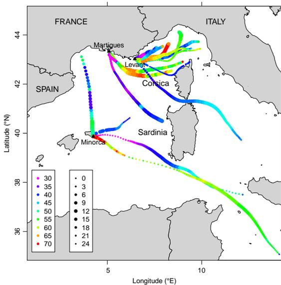
**Figure 9.** Trajectories of the 16 ozone BLPB flights launched in 2012 and 2013. The colour code (left box) represents the ozone mole fraction (in ppbv) measured along the trajectory. The dot size represents the solar local time (right box).
