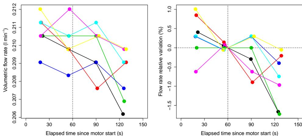
**Figure 6.** Pump flow rate evolution after sonde motor restart ( $t = 60$  s corresponding to the beginning of the measurement phase). Each data series is differentiated with colours. **(a)** Volumetric flow rate ( $\text{L min}^{-1}$ ). **(b)** Relative deviations (in %) from the flow rate interpolated at  $t = 60$  s after restart.
