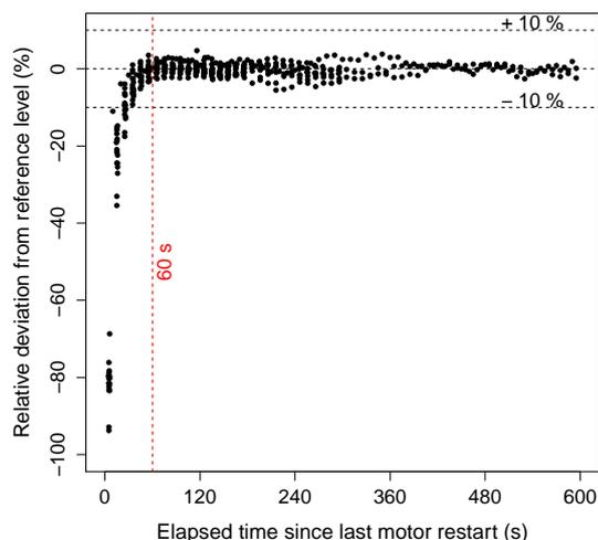
**Figure 5.** 12 May 2011 ground-based experiment. Deviation of  $S_{\text{Exp}}$  data from the values predicted by the linear model (in relative value with respect to  $S_{\text{Ref}}$  data), as a function of time elapsed since the last restart of the motor. The red dashed line marks 60 s (warm-up time adopted thereafter). The horizontal dashed lines mark deviations of  $-10\%$ ,  $0$  and  $+10\%$ .
