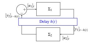
Fig. 2. Feedback interconnection of two PHSs with time-varying delay.
