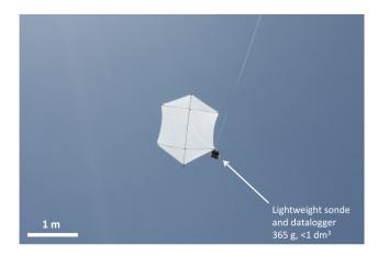
**Figure 2.** View of the rokkaku kite and lightweight sonde and data logger assembly used for lidar calibration.
