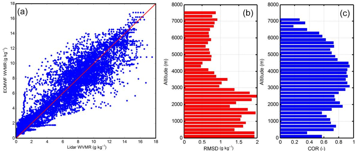
**Figure 6.** (a) Scatter plot between ECMWF and lidar-derived WVMR over all simultaneous measurements (blue dots). The red line is the identity. (b) Root mean square difference and (c) correlation between simultaneous profiles as a function of altitude (RMSD and COR as defined in the text).
