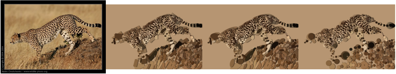
Figure 5: Shape selection and single shape rendering. The background of the original image, from www.wildlife-photo.org courtesy of Vadim Onishenko (left), is eliminated using a segmentation procedure [Felzenszwalb and Huttenlocher, 2004], the resulting image's colored tree is filtered using a contrast based automated procedure [Desolneux et al., 2001]. All the shapes from the resulting sketch are replaced with (from left to right) rectangles, ellipses, or disks.
