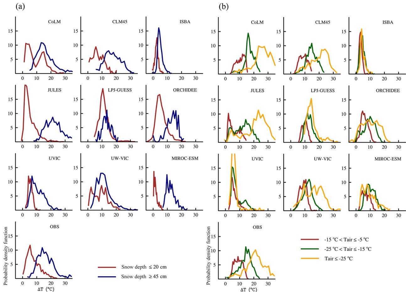
**Figure 2.** Conditional probability density functions (PDFs) of  $\Delta T$  ( $^{\circ}\text{C}$ ), the difference between soil temperature at 20 cm depth and air temperature for (a) different snow depth classes and (b) air temperature regimes for winter 1980–2000.
