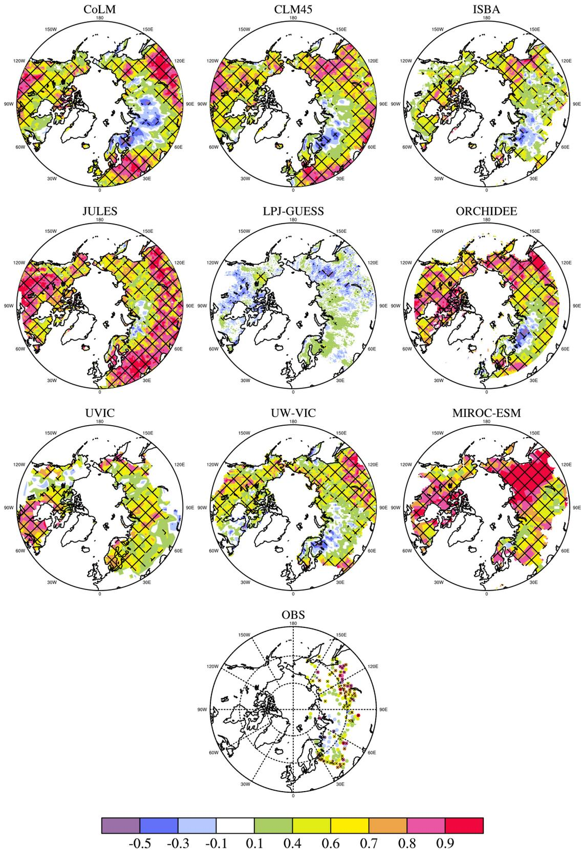
**Figure 3.** Spatial maps of the correlation coefficients between snow depth and  $\Delta T$ , the difference between soil temperature at 20 cm depth and air temperature for winter 1980–2000. Regions with greater than 95 % significance are hashed.
