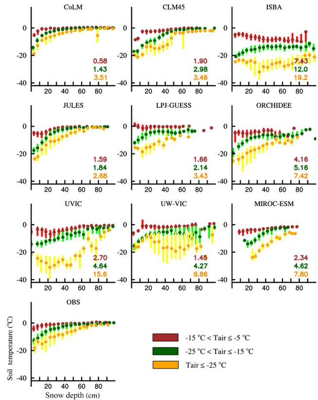
**Figure 5.** Variation of soil temperature at 20 cm depth (°C; y axis) with snow depth (cm) for winter 1980–2000. The dots represent the medians of 5 cm snow depth bins and the upper and lower bars indicate the 25th and 75th percentiles, calculated from all Russian station grid points ( $n = 268$ ) and 21 individual winters. The numbers in each model panel indicate the RMSE between the observed and modelled relationship. Colours represent different air temperature regimes.
