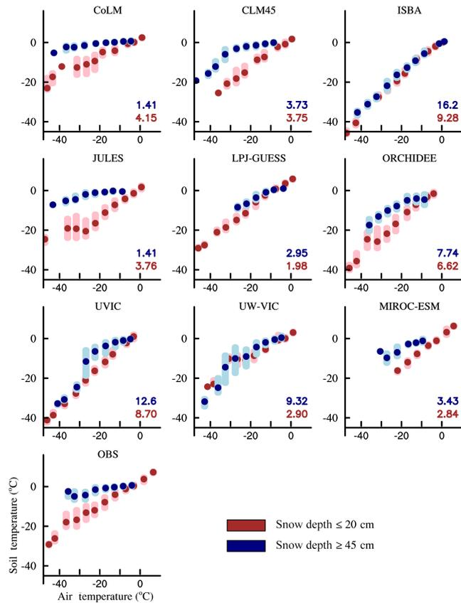
**Figure 4.** Variation of soil temperature at 20 cm depth (°C) with air temperature (°C) for winter 1980–2000. The dots represent the medians of 5 °C air temperature bins and the upper and lower bars indicate the 25th and 75th percentiles, calculated from all Russian station grid points ( $n = 268$ ) and 21 individual winters. The numbers in each model panel indicate the RMSE between the observed and modelled relationship. Colours represent different snow depth regimes.
