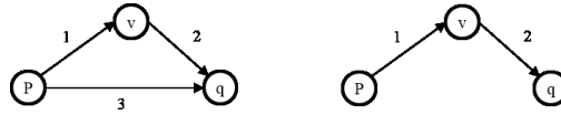
Figure2: removing an unnecessary transfer edge (p,q) since there is a better alternative via the node v
