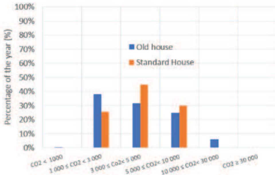
Figure 12- CO 2 concentration distribution in the building for the year, for an injection flux of 0.01 kg/s, a vadose permeability of 5.10^{-11} m 2 , a slab permeability of 2.10^{-13} m 2
