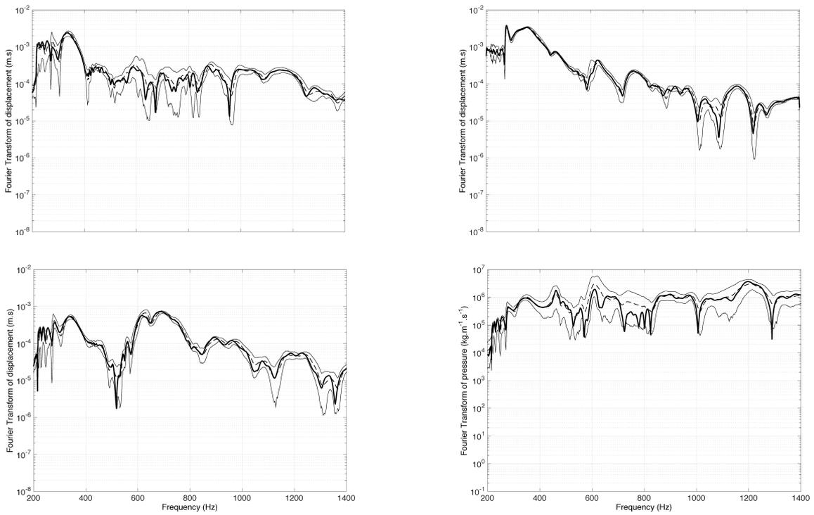
Figure 3: For  $\delta_{K_F} = 0.2$ , graph of the deterministic response (thick line), the mean response (thin dashed line) and of the confidence region related to (a) displacement  $\tilde{U}_x(\nu)$ , (b) displacement  $\tilde{U}_y(\nu)$ , (c) displacement  $\tilde{U}_z(\nu)$ , (d) pressure  $\tilde{P}(\nu)$ .
