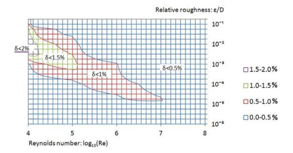
W solutions of CW equation for flow friction
