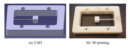
FIGURE 2 – CAO and 3D printing of the test structure.
