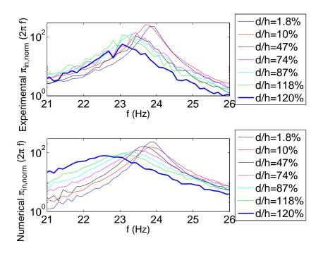
Figure 6 – Comparison of the experimental normalized input power density  $\pi_{\text{in,norm}}^{exp}$  with the identified computational model for the seven amplitudes.
