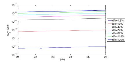
FIGURE 4 – Experimental PSD function  $S_{F_x}^{exp}$  for seven amplitudes of the excitation.
