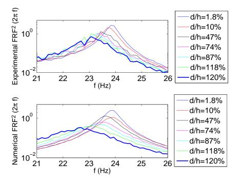
FIGURE 5 – Comparison of the experimental  $FRF^2$  (exp) with the identified computational model (num) for the seven amplitudes.
