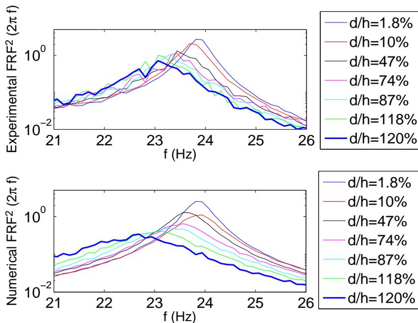
FIGURE 5 – Comparison of the experimental FRF<sup>2</sup> (exp) with the identified computational model (num) for the seven amplitudes.
