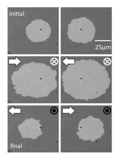
**Figure 4.** Bubble shifting by magnetic fields. Sequence of direct Kerr images showing the bubble shifting in the  $Pt_{30}Co_6Pt_{18,7}$  sample by combined in-plane and perpendicular fields  $(H_{ip} = 40 \text{mT} \text{ and } H_z = 11 \text{mT})$  The relative direction of the in-plane and perpendicular magnetic field is indicated on the images. The same experimental parameters are used in the supplementary movie.
