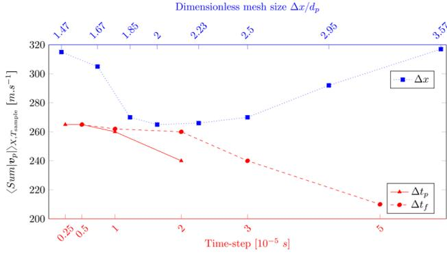
**Figure 9.** Influence of solid time-step magnitude (red line), fluid time-step magnitude (red dotted line), and fluid grid size (blue dotted line) on the time-averaged sum of all particles velocity norm, selected as a major feature of the computed solution.
