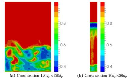
**Figure 10.** Snapshots at  $t = 2.8$  s of the fluid volume fraction spatial distribution in a homogeneous bubbling fluidized bed in a vertical cut plane for domains with (a) a wide cross section and (b) a narrow cross section.
