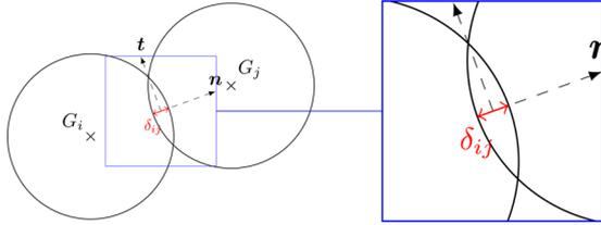
**Figure 1.** Contact between two particles:  $G_i$  and  $G_j$  denote the centers of mass of particles  $i$  and  $j$ , respectively,  $M$  the contact point,  $\mathbf{n}$  and  $\mathbf{t}$  the unit normal and tangential vectors at the contact point, respectively, and  $\delta_{ij}$  the overlapping distance.
