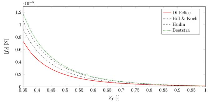
**Figure 2.** Drag force depending on the fluid volume fraction for a particle of diameter  $d_p = 10^{-3}$  m with a relative velocity  $|\mathbf{u}_f - \mathbf{v}_p| = 0.35$  m/s in air ( $\rho_f = 1.2$  kg/m<sup>3</sup>,  $\mu_f = 1.8$  Pa s). Correlations proposed by Di Felice,<sup>15</sup> Hill and Koch,<sup>17</sup> Huilin,<sup>34</sup> and Beetstra.<sup>18</sup>
