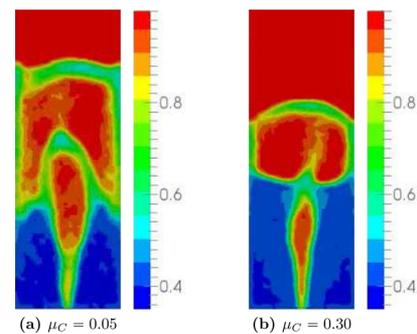
**Figure 18.** Snapshots at  $t = 1.5 \text{ s}$  of the fluid volume fraction spatial distribution for two different values of the tangential friction coefficient  $\mu_C = 0.05$  and  $\mu_C = 0.3$  in the single-nozzle spouted bed.
