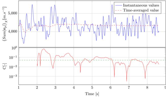
**Figure 8.** Time evolution of  $\langle \text{Sum}|\mathbf{v}_p| \rangle_X$ , its time average  $\langle \text{Sum}|\mathbf{v}_p| \rangle_{X, T_{\text{sample}}}$  (above) and the convergence criterion  $C(T_{\text{sample}}, T_{\text{var.}})$  (below).
