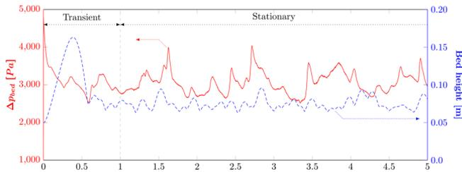
**Figure 7.** Time evolution of the bed height (dashed blue) and of the dynamic pressure drop across the bubbling bed (solid red).
