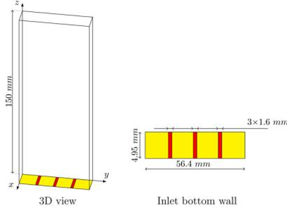
**Figure 14.** Domain geometry of the spouted bed experiment used by Brown.<sup>44</sup>
