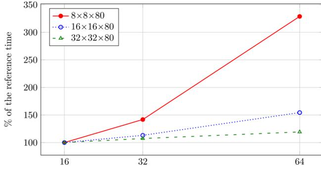
**Figure 6.** Evolution of the scaling performance for the solution of the Stokes problem as a function of the number of cores for different fluid cells loads per core. The reference is the time spent on a full node (16 cores).
