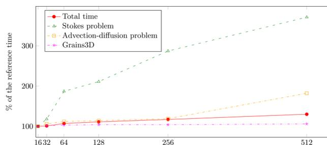
**Figure 5.** Scaling performance for a constant load per core (80,000 particles/5120 fluid cells). Evolution of the computational time spent in the various parts of the code as a function of the number of cores normalized by the time spent on a full node (16 cores).
