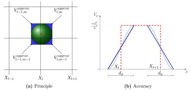
**Figure 4.** Our embedding cube/square approximation method: (a) principle and (b) accuracy of the approximation as the evolution of particle volume crossing control volume  $l$ : (green dots) disc analytic solution, (blue line) our embedding square approximation method, (red dotted line) particle center method.
