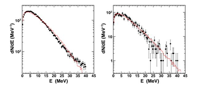
Figure 2. Particle spectra from  $N_a$  sources: <sup>16</sup>O\* (left) and <sup>28</sup>Si\* (right). Black dots with statistical error bars correspond to experimental data. Histograms superimposed on data correspond to filtered simulations of a simultaneous decay process (see text).
