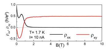
FIG. 1. Magnetoresistance observed in sample G31 at low temperature T=1.7 K and low current I=10 nA. A quantum Hall plateau at  $\rho_{xy}=R_K/2$  initially develops when B increases up to 0.5 T. At higher B, the Hall resistance changes sign and a long plateau appears at  $\rho_{xy}=R_K/2$ . The longitudinal resistance  $\rho_{xx}$  shows a pronounced maximum when the Hall resistance changes sign.  $\rho_{xy}<0$  (>0) corresponds to holes (electrons).
