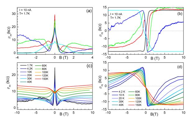
FIG. 4. (a) Longitudinal and (b) transverse magnetoresistances observed in sample G14 at T = 1.7 K and I = 10 nA. The different curves correspond to five different sample preparations, indicated by the colored squares in Fig. 2. (c) and (d) Temperature dependence of the longitudinal and Hall magnetoresistances ( $\rho_{xx}$  and  $\rho_{xy}$ ) for an additional sample preparation, close to the red square in Fig. 2.
