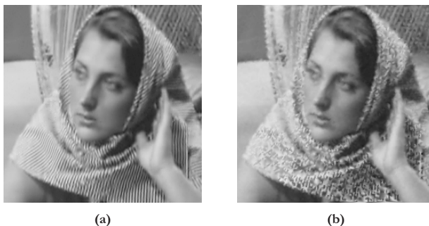
FIGURE 18. Restoration of the “Barbara” face image: (a) using patch-based DST regularization with the Geman and McClure potential (SSIM = 0.87376, PSNR = 25.847 dB); (b) using cubic interpolation (SSIM = 0.75858, PSNR = 21.631 dB).
