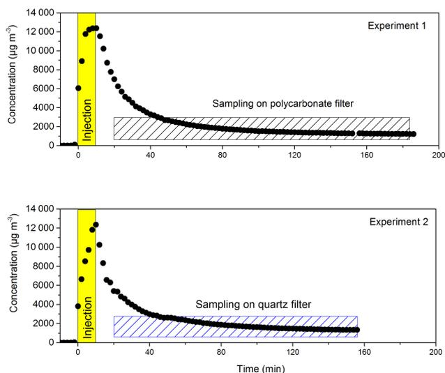
**Figure 1.** Time series of aerosol mass concentration in the chamber for two companion experiments (Libyan dust). Experiment 1 (top panel) was dedicated to the determination of the chemical composition (including iron oxides) by sampling on polycarbonate filters. Experiment 2 (bottom panel) was dedicated to the determination of the absorption optical properties by sampling on quartz filters.
