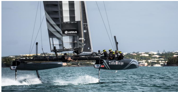
FIGURE 1. Principle of the flying boat with the AC45 of Oracle USA Team - TV snapshot
