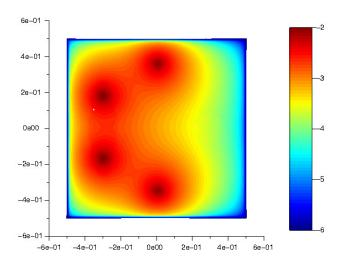
Fig. 2. Sum of  $\log_{10}$  of initial condition of Wave equation (2) for 4 sources distributed on the left  $(\sum_{k=1}^{s} (\log_{10} \Gamma \mu_a \Phi^k + 10^{-6}))$ .
