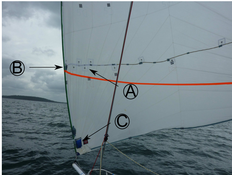
Figure 2. Photograph of the spinnaker tack. (A): tack shackle wired to the acquisition box. (B): wire running along the foot from the clew shackle to acquisition box. (C): Acquisition box with strain gauge amplifiers, a microcontroller, a wireless transmitter and a battery.
